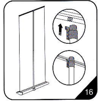
16. The plastic holder at the top of pole slips into the rear slot of the banner beam. A marker on the beam indicates the beam's centre where the pole should be inserted.
